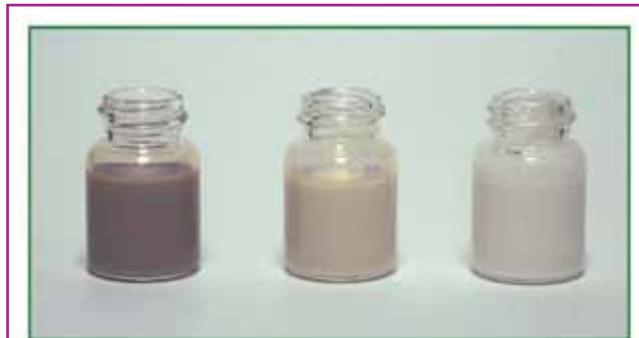
Figure 2. (The visible colour change of 10 nm, 15 nm, and 60 nm particle size dispersions of titanium dioxide when combined with ascorbyl palmitate).
