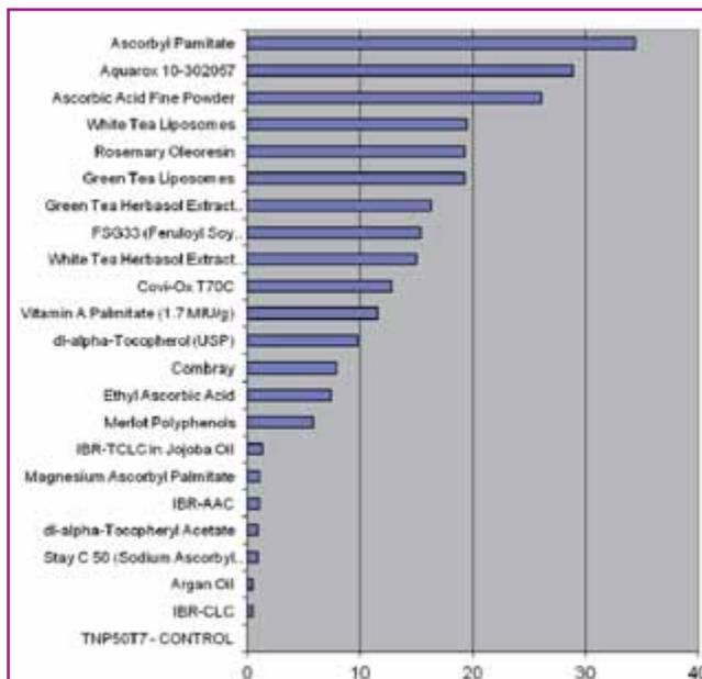
Figure 3. Antioxidants effect on colour change of a titanium dioxide dispersion CIELAB Colour difference after 5 days at room temperature.
